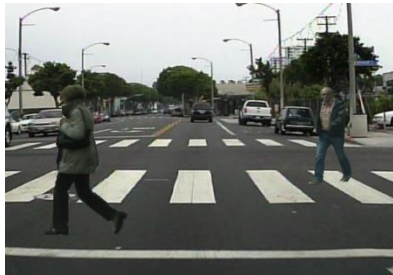
Synthetically placed pedestrians using the cut-and-paste method on road ground plane.
